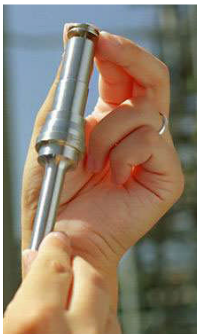
Figure 1.7 The BASIL process is run in a small jet reactor. The plant has a total capacity of 690\,000\text{ kg m}^{-3}\text{ h}^{-1} . 25
