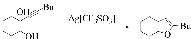
Scheme 4.10 Synthesis of 2-butyl-4,5,6,7-tetrahydrobenzofuran catalysed by silver triflate.
