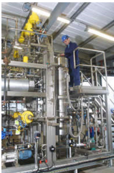
Figure 1.14 Thomas Swan plant for the use of supercritical fluids as solvents. 82
