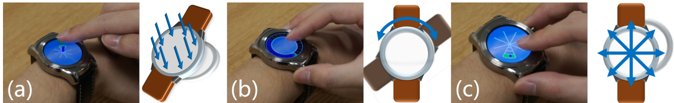
Figure 1. The three main techniques proposed in our paper: (a) Omni-direction pressure touch (b) Bi-direction twist and (c) Omni-direction panning.
