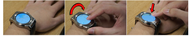
Figure 5. Map application running on LG watch Urbane: Twist to zoom and pressure touch to move the map at different speed.
