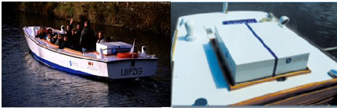
Figure 1.7: (a) Hydra, boat with fuel cell propulsion. It's a cruise boat 12 m long, with 6.5 kW AFC fuel cell, which has a capacity of twenty two passengers plus one skipper. (b) Alkaline Fuel Cell [22, 23]
