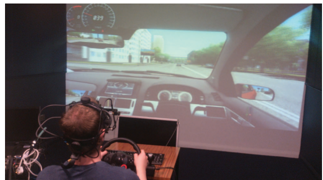
Figure 1. The basic experimental setup. Participants wore an eye tracker and were seated in front of a calibration screen and main projection screen. See the online article for the color version of this figure.
