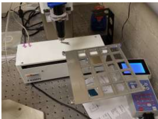
Figure 4. Holder plate with space for 20 array mounts. Positional accuracy was specified to be better than 200 \mu m in x & y.
