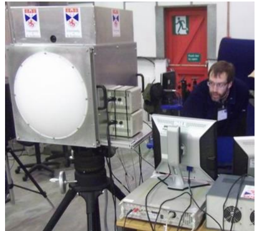
Figure 1: IRAD 340 GHz radar undergoing field trials.
