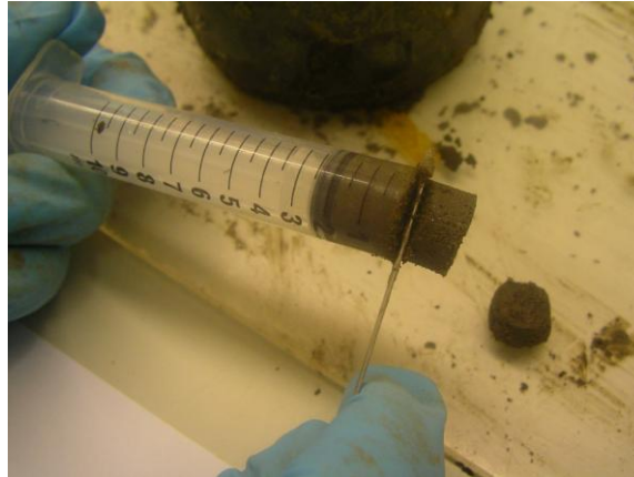
Figure 4.3. The course corer, with sediment pushed out of the core and cut to the desired depth.
