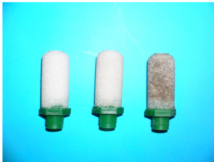
Figure 3.7. Three Mark IV CSM filters, (a) new, (b) moderately used and (c) heavily used.
