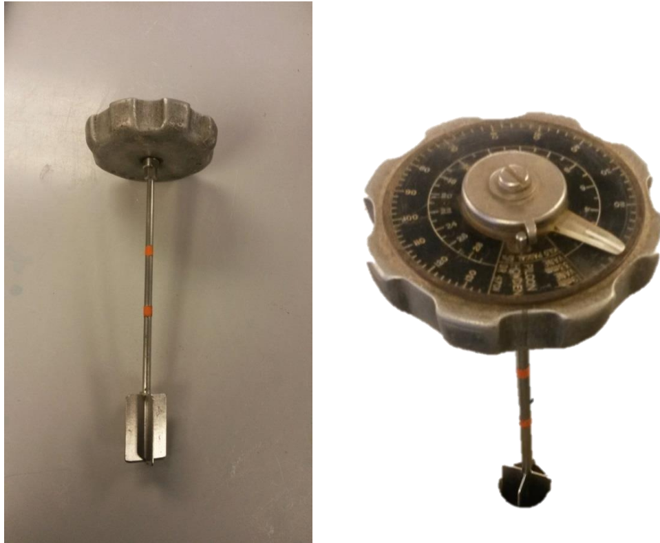
Figure 2.4: Shear Vane: for use in measuring the shear strength of sediment
