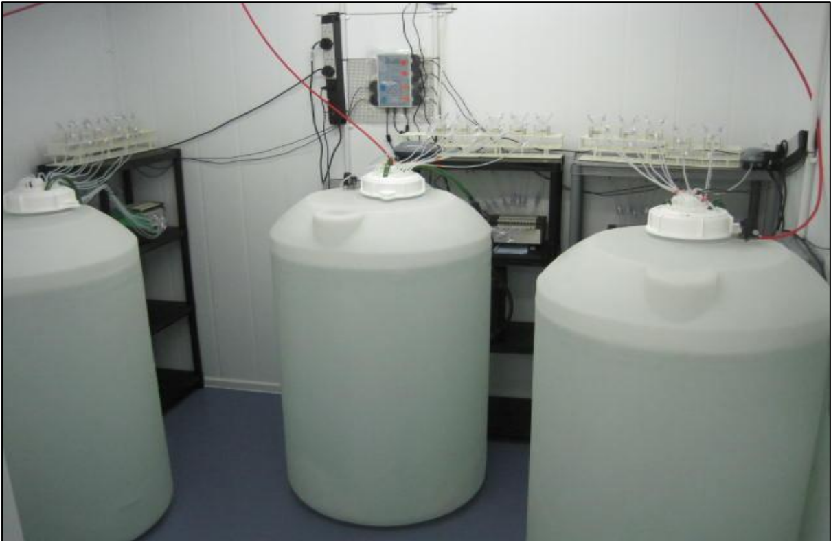
Figure 2.4 Photograph of culturing system showing the reservoir tanks, culture chambers and carbonate chemistry manipulation system.
