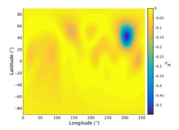
**Figure** 6. The density perturbation,  $\rho_m = r^2 [\xi'(r)(r \cdot B)^2/2 + r\xi(r)B \cdot \nabla(r \cdot B)]$ , at the stellar surface. Values on the colour scale are non-dimensional as specified in equation (4).
