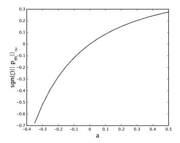
**Figure 2.** The variation of the signed maximum magnitude of the pressure perturbation  $p_m$  as a function of a for fixed  $\alpha$ =0.3. Values on the axes are non-dimensional as specified in equation (4).
