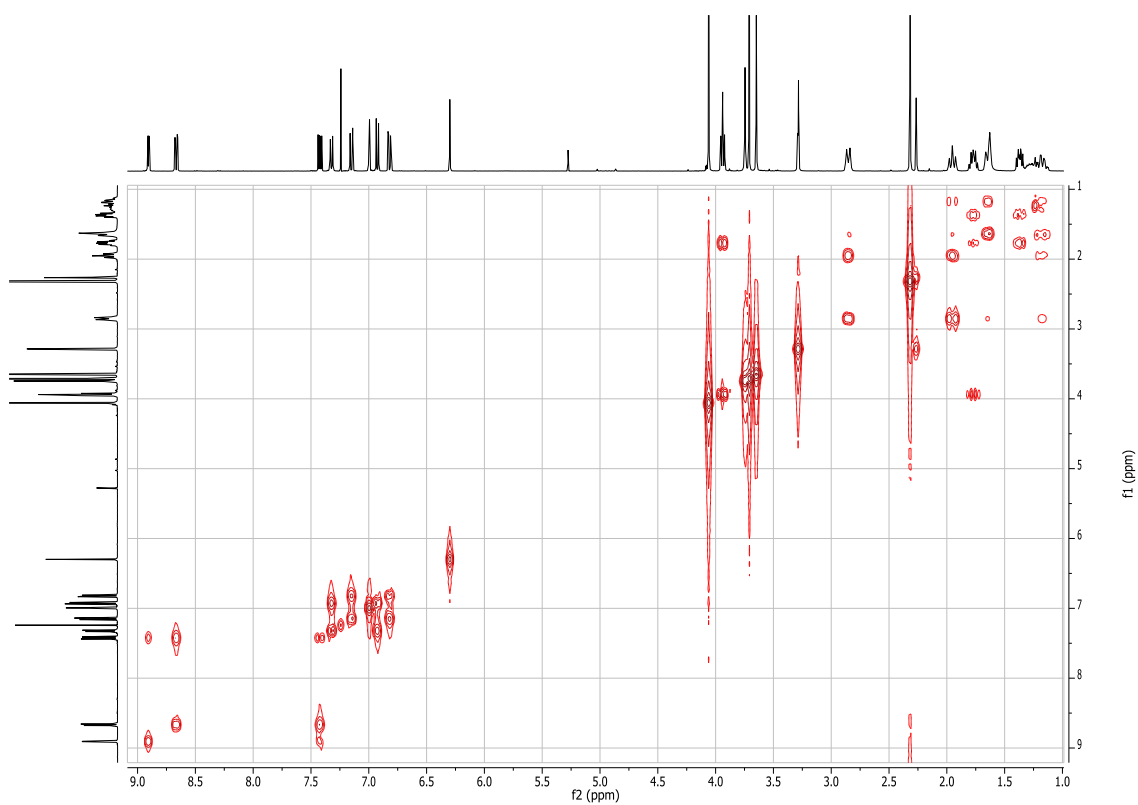
^1\text{H} - ^1\text{H} g-COSY (400 MHz, \text{CDCl}_3 ) spectrum of compound 4 .
