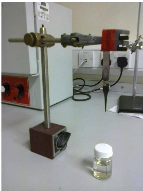
Figure 23: Apparatus aimed to half-dipping operation. The clamp can be moved up and down to partially immerse the sample in the incubation vial full of 100 \mu\text{M} \text{PdSO}_4 solution, located beneath the clamp itself.
