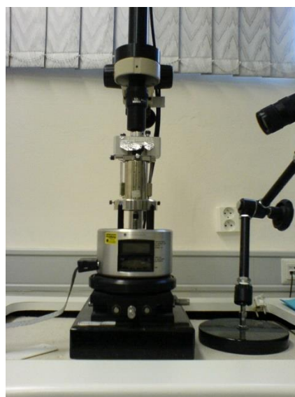
Figure 12: Example of AFM apparatus. The sample is put in the chamber, at half of the height of the apparatus.
