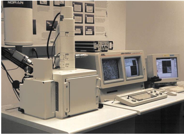
Figure 9: Image of an SEM apparatus. The microscopy chamber on which the electron column sits is seen on the left.
