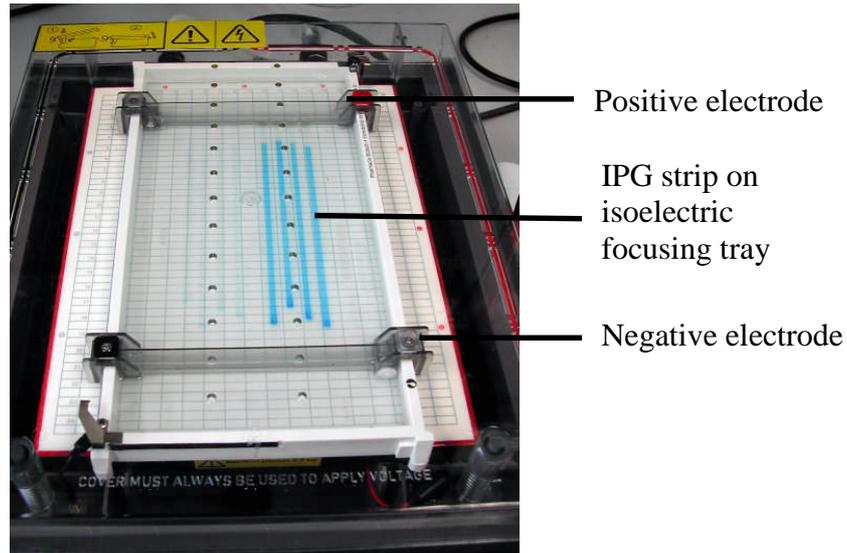
**Figure 2.1: MultiphorII isoelectric focusing unit.**
