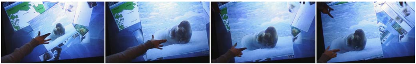
Figure 15. Item is enlarged by spreading thumb and middle finger and, using these same two touch points, the item is dragged towards the participant.
