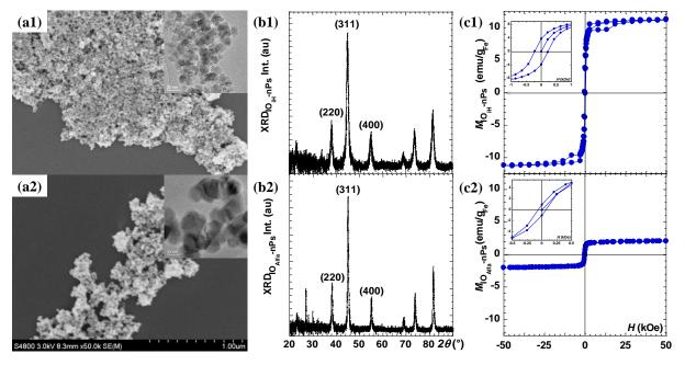
**Fig. 1:** For IOiH-nPs (1) and IOAlfa-nPs (2): Scanning Electron Microscopy images (a), XRD spectra of the Fe<sub>3</sub>O<sub>4</sub> nPs (b) and hysteresis curves completed at room temperature (c). Insets present TEM images of IO-nPS with a 20 nm scale bar (a) and zoomed magnetisation response for low magnetic fields (c).
