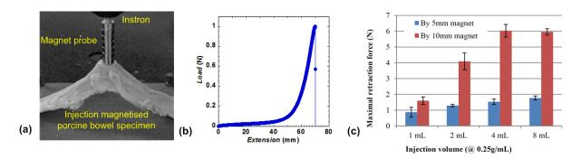
**Fig. 2:** Ex-vivo porcine bowel retraction and force measurement: (a) Photograph of a magnetised bowel segment retracted during Instron force measurement. (b) Extension-load curve demonstrating a maximum force before slipping occurs (normalised to unity for illustration purpose). (c) Injection volume versus magnetic retraction force using two-sized magnet probes.
