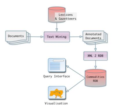
Figure 5: Trading Consequences System Architecture.
