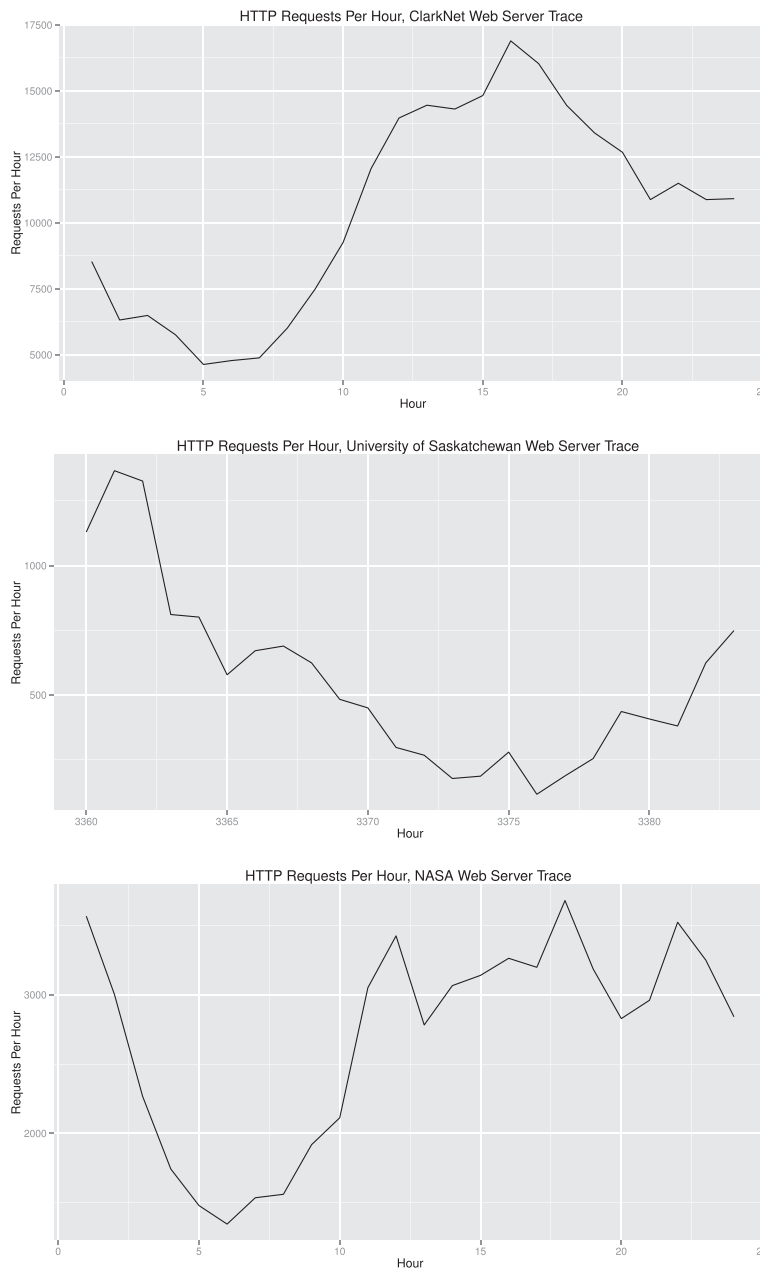
Fig. 12 Examples of traces of HTTP requests per hour over a 24 h period. Taken from a number of common public sources. Shown here are traces from the University of Saskatchewan, NASA and ClarkNet
