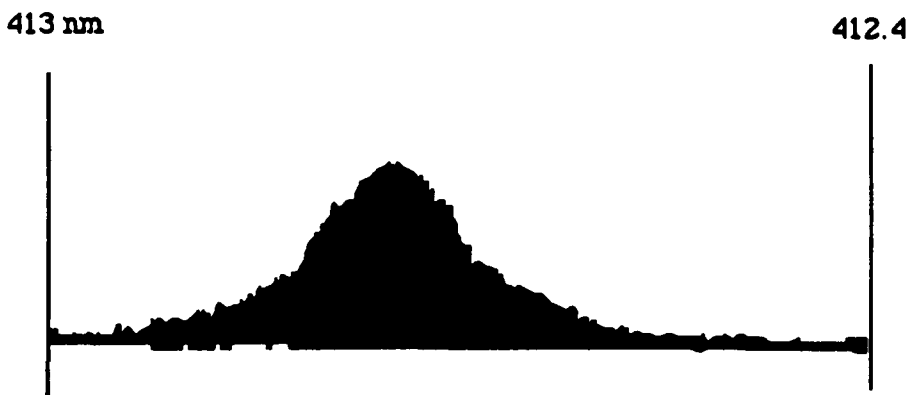
Figure 4.24. Spectrum of yzLBO at 40°. The FWHM linewidth is 0.15 nm.
