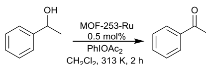
Scheme 1.12: Oxidation of 1-phenylethanol to form acetophenone in dichloromethane catalysed by MOF-253-Ru
