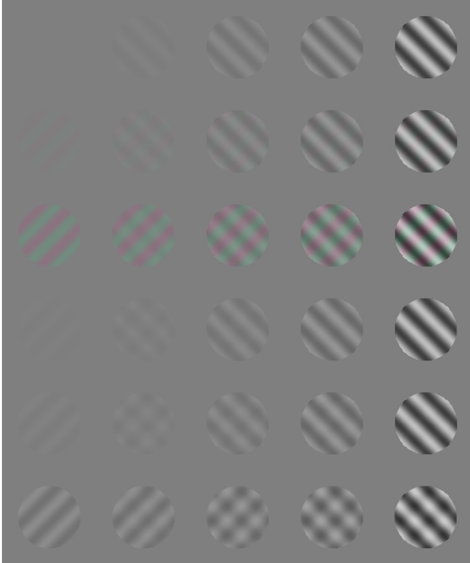
Figure 6.1: Representations of the 30 conditions used in the experiment. The order of the stimuli follows Table 6.2. Participants were asked to match the right oblique luminance component in all stimuli. The contrast adjustable matching stimulus was similar to the baseline stimuli (first row).
