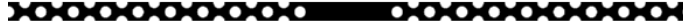
Fig. 8.2: Schematic of the supercell used to model the band-structure of a W3 waveguide in MPB
