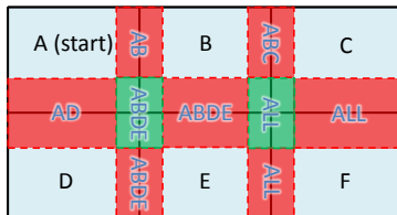
Figure 5. Window manager behavior for a drag on a window that occupies tile A. The letters in each area indicate the tiles where the window will be moved/expanded if a drag starting in A ends in that area.
