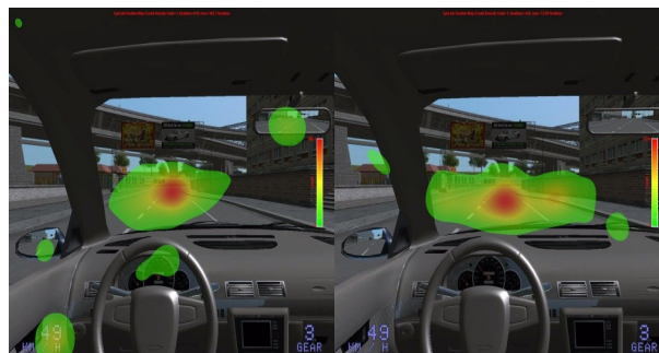
Figure 2. Example (from one observer) of density heat maps showing the distribution of fixations for the Driving (left) and Non driving (right) condition where red represents a greater proportion of fixations.
