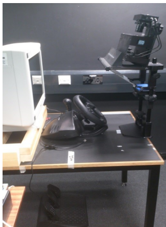
Figure 1. Apparatus set up of monitor (left), steering wheel and pedals and eye tracker (right)
