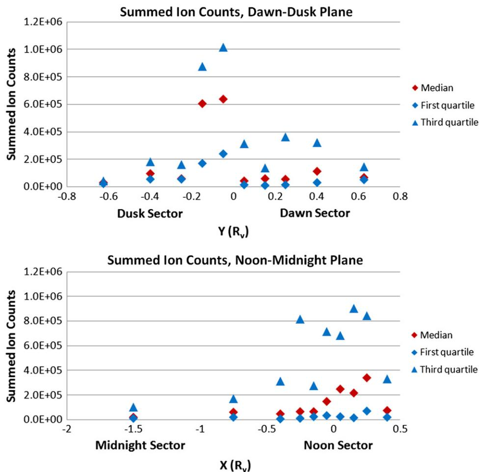
**Fig. 3.** Summed ion counts in a narrow plane aligned dawn–dusk (upper panel) and in a narrow plane aligned noon–midnight (lower panel) between 4th August 2008 and 17th March 2009 as a function of distance from the pole of the planet. Observations below the ICB for which the  $x$  coordinate is  $|x| < 0.2 R_v$  were used for the dawn–dusk plane and observations below the ICB for which the  $y$  coordinate is  $|y| < 0.2 R_v$  were used for the noon–midnight plane.
