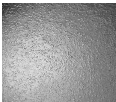
Fig 2.29. A seeding experiment drop with very small crystals of the 5-FDRPi due to over-nucleation.
