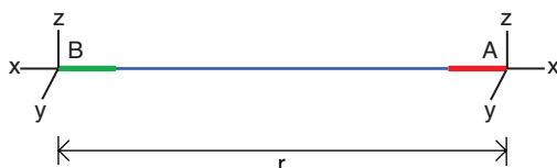
Figure 3.2.1. A semi-rigid nitroxide biradical described by a vector model. The blue vector represents the rigid molecule. The red and green vectors represent the nitroxide moieties and their flexible linkers (spin labels A and B). The relative orientation of nitroxides A and B is described by the unit vectors, x, y, z. The interspin vector r between the spin centres is shown by the black vector below.
