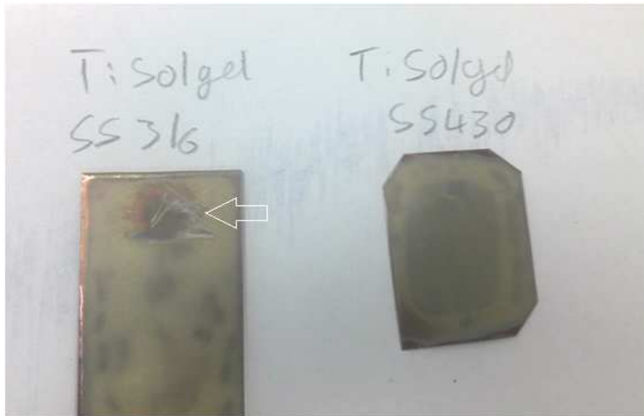
Fig.5.9: SS430 and SS316 with acidified alcohol sol-gel solution painted and fired at 400°C for 24 hours. Scratch mark denoted by white arrow.
