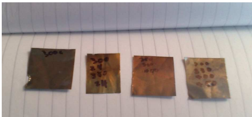
Fig.5.20: SS430 samples coated with titanium by sputtering fired for increasing durations at increasing temperatures.
