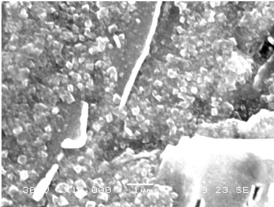
Fig.6.15: SS430 coated with thick cobalt and heated for 3 days at 700°C
