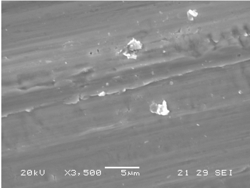
Fig.6.2: SS430 coated with Co without heat treatment
