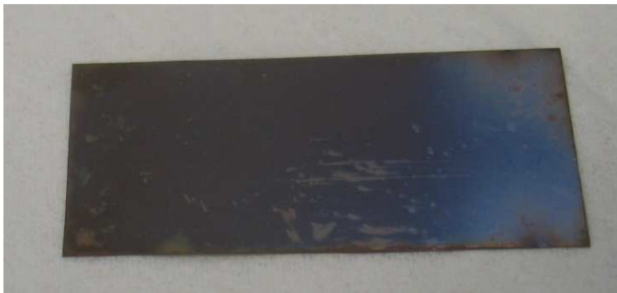
Fig.5.38: Back side of sample from fig.25 showing corrosion.
