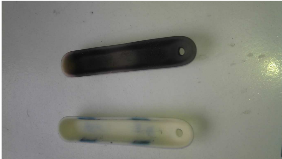
Fig.4.8: Sample boats. Top was \text{Cr}_2\text{O}_3 in wet \text{O}_2 at 1200C, bottom was spinel for same conditions.
