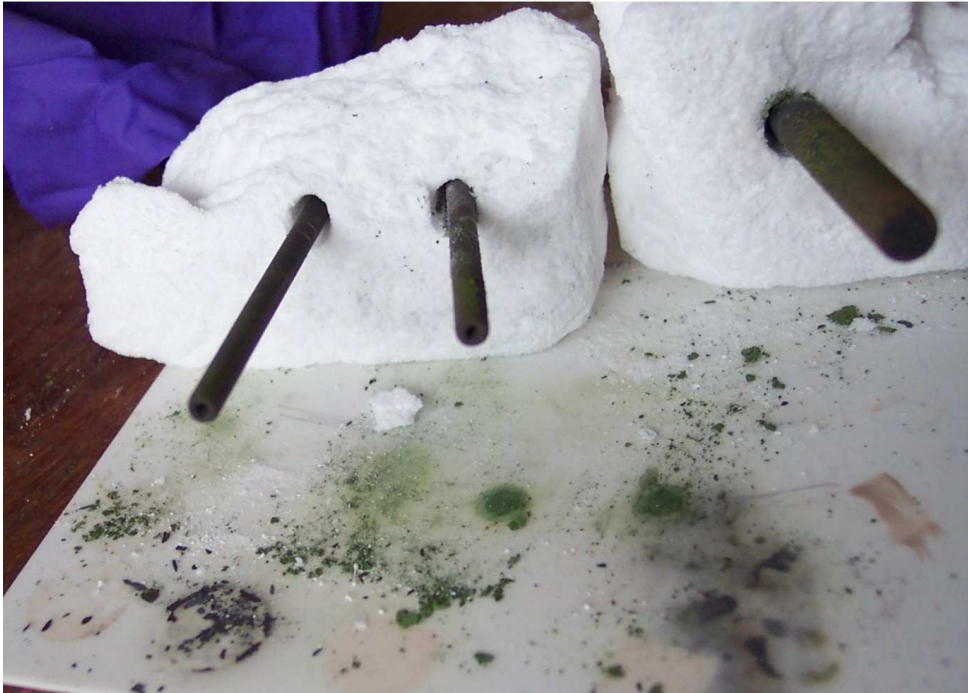
Fig.5.3: Stainless steel pipes and rod coated with CTO sol-gel and fired at 900C. The resulting CTO powder can be seen on the alumina plate below. Powder that remained in the pipes and rod brushed off with ease.
