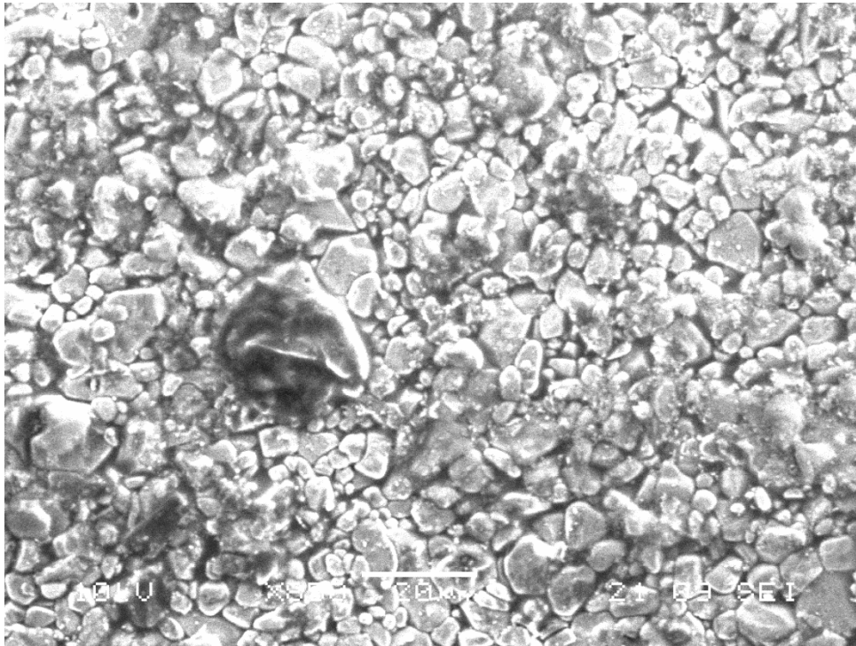
Fig.5.17: SEM of Sample from Fig.5.15a, Ti metal on Alumina.
