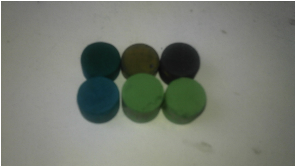
Fig.4.9: Pellets colour change: left to right, Spinel, CTO, Cr203. Top row post ox, bottom row pre oxidation
