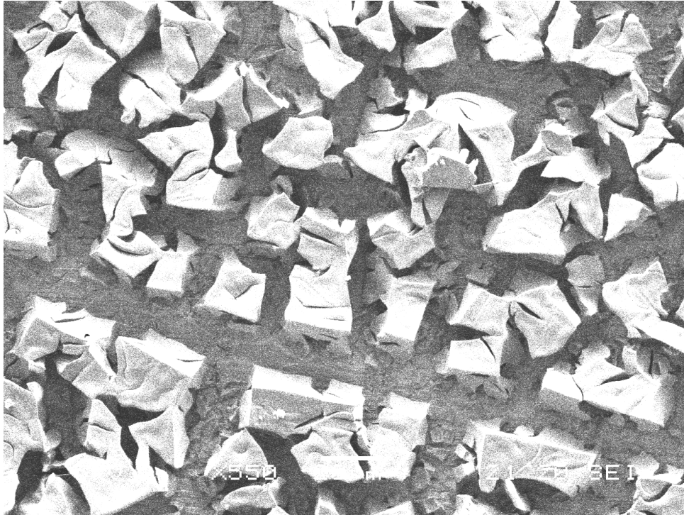
Fig.5.11: SEM of acidified alcohol based Ti sol-gel
