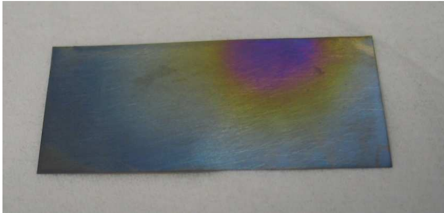
Fig.5.39: SS430 with Ti after 15 days at 400°C
