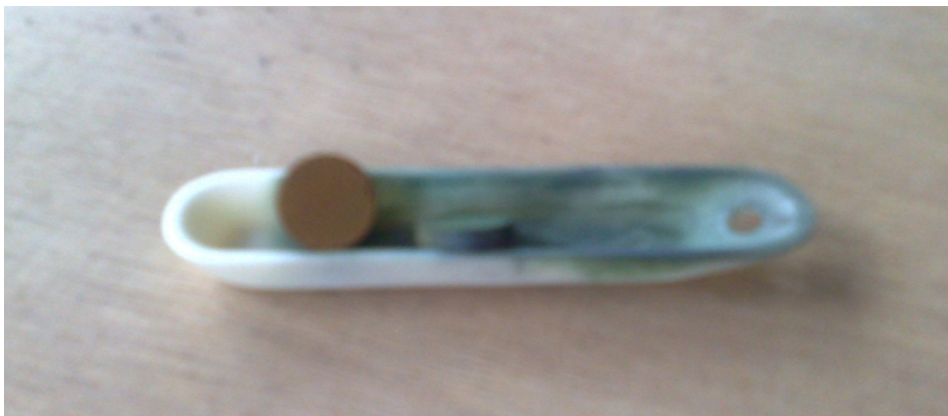
Fig.4.7: showing CTO evaporation sample. Flow was from left to right.
