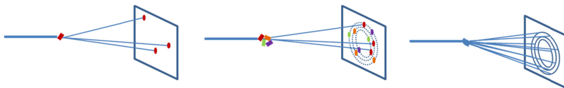
Figure 3-16: Schematic showing the diffraction spots from a single crystal (left), several crystallites (middle) and diffraction rings from a crystalline powder (right).
