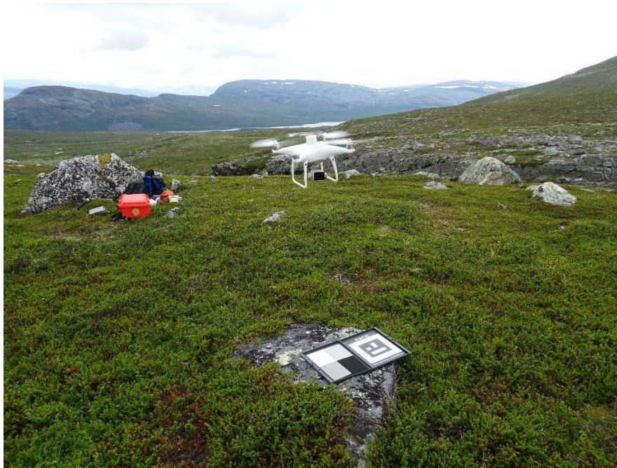
Fig. 43 Multispectral UAV and reflectance target used for the aerial survey.
