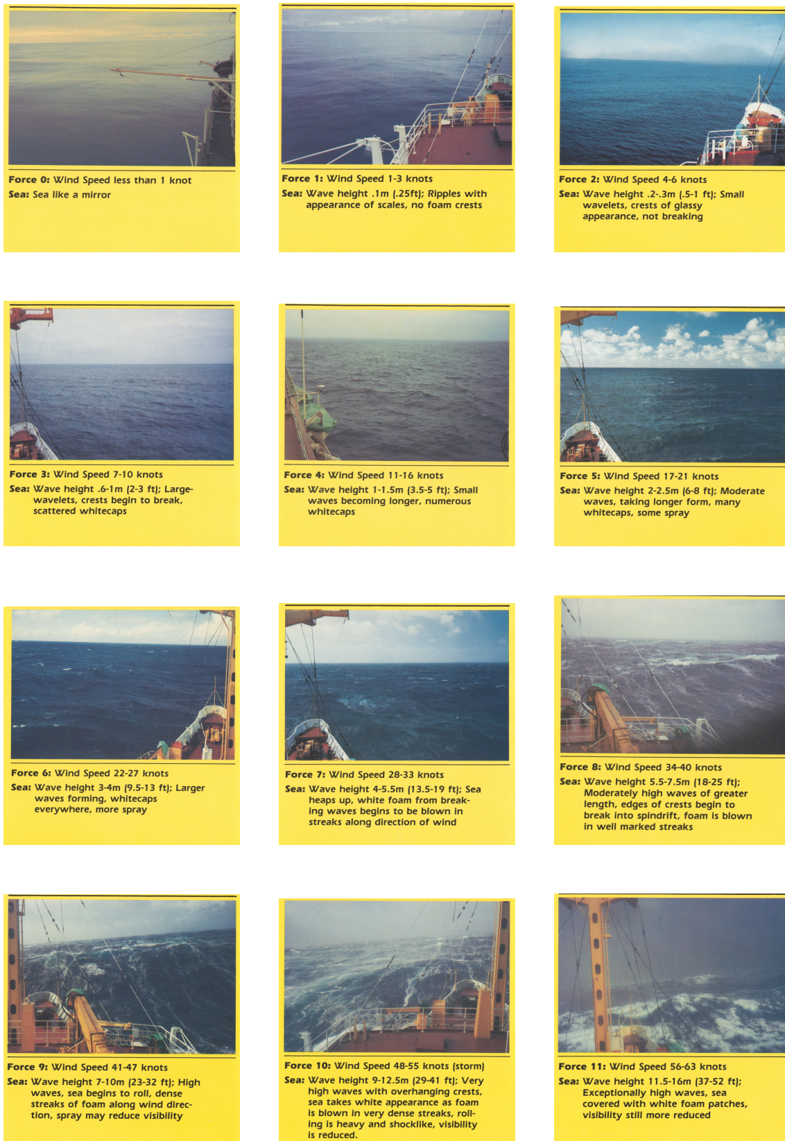
Figure 2.12: The Beaufort wind scale. Adapted from the National Oceanic and Atmospheric Administration [69].
