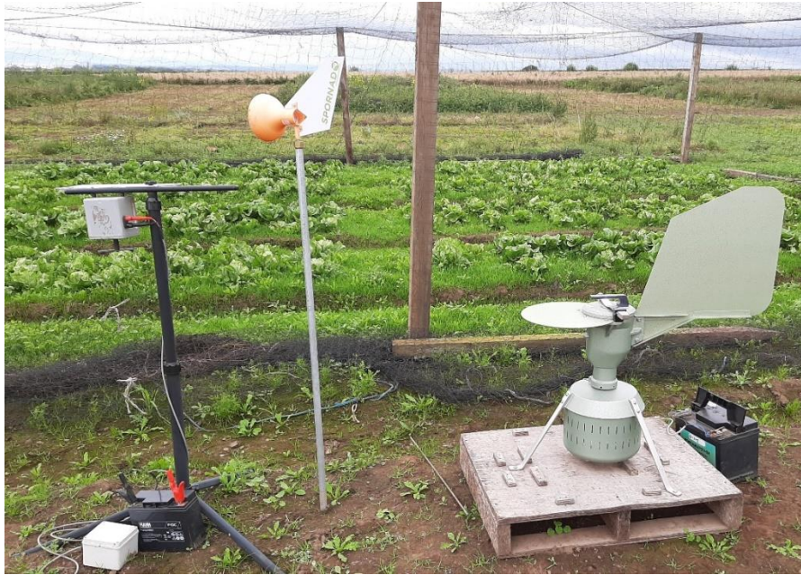
Figure 5-6 Aerial samplers at the 5m (H3 position) from the centre of the field trial. The GRIPS-99M (H3 5 m) aerial sampler (left), the Burkard 7-day continuous samples (Tape trap) (right).
