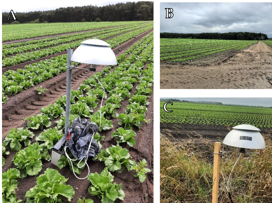
Figure 5-7 Rotorod sampler at commercial field sites. A: Rotorod sampler with rain guard attached. B: Scottish field site 2 (2021), and C: English field site 1 (2021).
