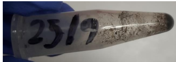
Figure 5-8 Example of Multivial sample collected, note the amount of soil contained.
