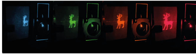
Figure 5.17 The obtained experimental efficiency at visible wavelengths regime, with the strip below showing and experimental holographic image at 488, 532, 590, and 632 nm. The error bars represent the standard deviation from 4 measured metasurfaces. The error bars reflect the impact of fabrication quality, including the precision in the exposure and development of the meta atoms. Taken from [129].
