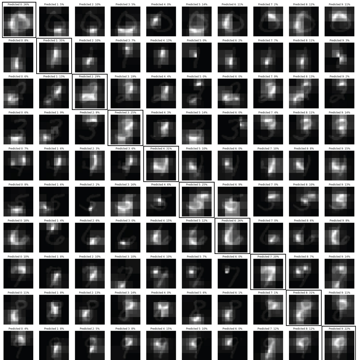
Figure 4.6: HiPe saliency on MNIST. Each row comprises saliency maps for each class on a single randomly chosen sample image. The top left to bottom right diagonal contains the saliency of the correct class for each sample. The probabilities shown here are the model output logits normalised to sum to one and rounded to the nearest percentage point.
