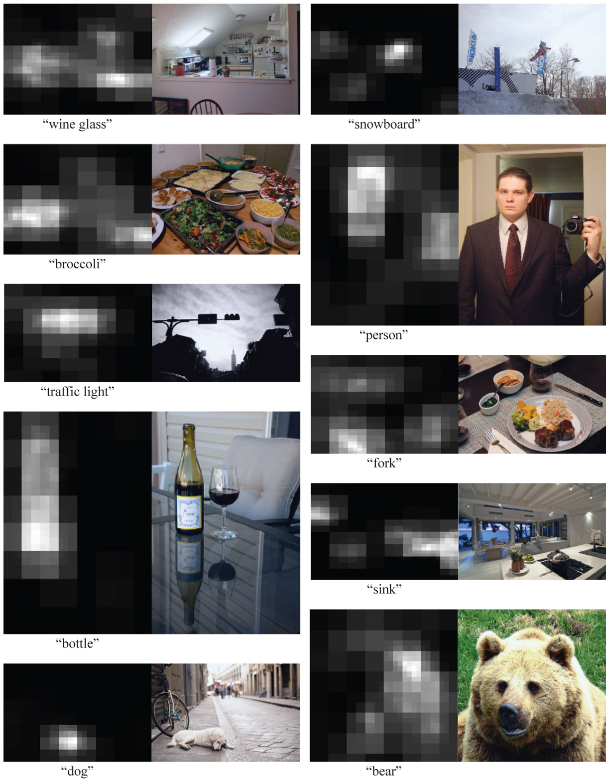
Figure 4.3: Examples of saliency maps generated with Hierarchical Perturbation. Note that more salient regions are of higher resolution - for example, for the "sink" class, the most salient region on the right has more finely-grained saliency than the less salient regions on the left.
