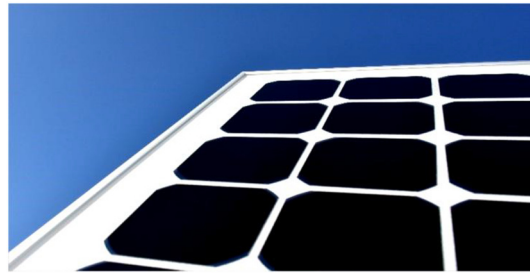
Fig. 4 Dry-etched black silicon IBC solar panel without any antireflection coating fabricated in Naps Solar Systems, Finland. The energy conversion efficiency of 18.1% and 19.9% of the whole IBC module and the best individual cell of the module, respectively, demonstrate that fragile nanostructures can withstand standard module fabrication steps. 65
