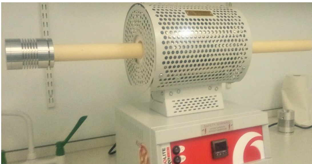
Figure 2-10: Carbolite Gero tube furnace in a dry room with a stainless-steel end with the lens allows for wetting reactions of metals to be seen at different temperatures.
