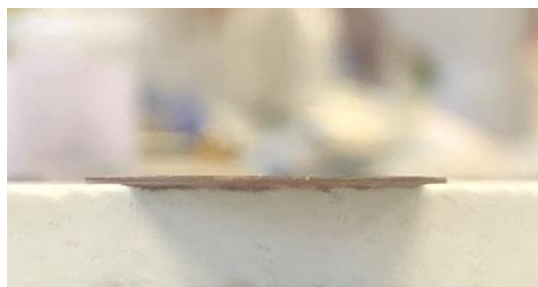
Figure 6-18. Sintered thick BCZY electrolyte tape.
