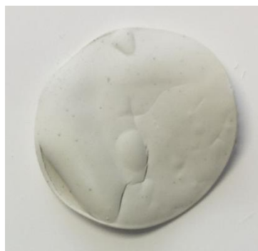
Figure 6-12 Typical sintered laminated tape at 1300 °C for 10 h.
