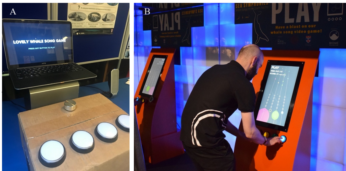
Figure 5.2.10: (A) The prototype version of the BIOME whale song game when being trialled at Explorathon 2019. The 4 buttons reflected different whale song units and the silver dial could manipulate the speed of the game. At this stage the game was called 'lovely whale song game'. (B) The final version of the BIOME whale song game installed in Dundee Science Centre.
