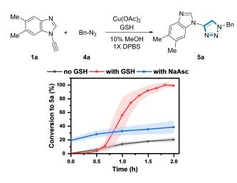
**Figure 3.** Influence of [GSH] and NaAsc on the formation of **5 a**. *Reaction conditions*: (black) **1 a** (200  $\mu$ M), **4 a** (500  $\mu$ M), Cu(OAc)<sub>2</sub> (350  $\mu$ M), 10% MeOH, 1X DPBS, rt. (red) + GSH (1 mM). (blue) + NaAsc (1 mM). Shaded error bands correspond to the standard deviation of three replicate experiments.
