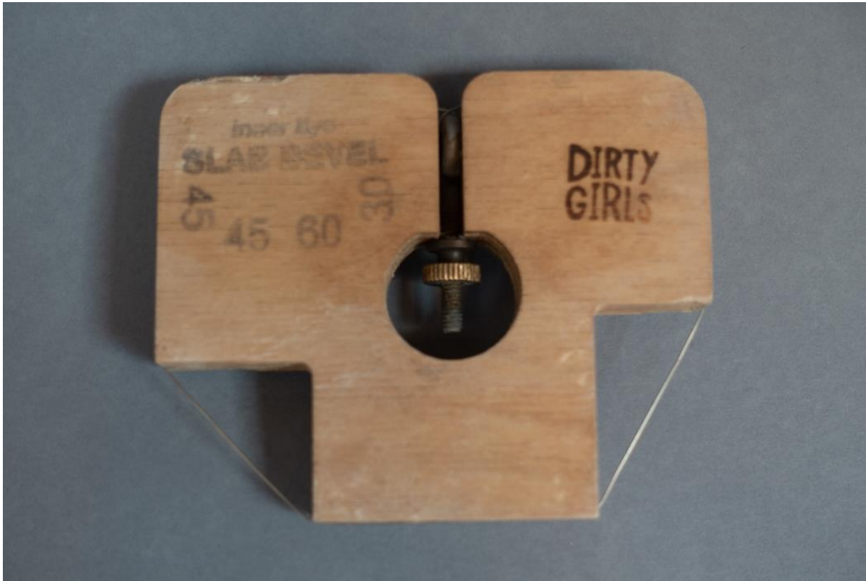
FIGURE 9. Tool for bevelling the edges of a slab of clay.
