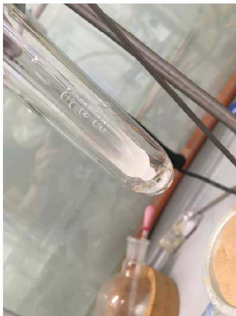
Figure 5.27 Sublimation apparatus with ( S )-2-fluorosuccinic acid ( S )- 315 solid on the cold finger.
