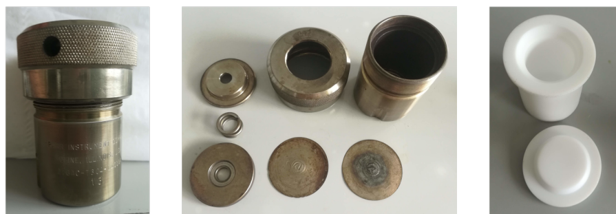
Figure 3.1. Photos of a fully assembled autoclave and its individual parts, including spring, pressure plates and a PTFE liner.
