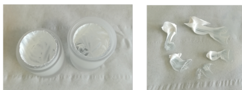
Figure 6.4. Photos of the milling jar after the reaction and the pasty product after scooping it out of the jar.
