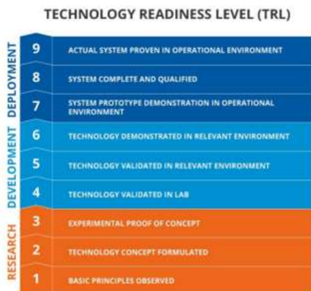
Figure 2: TB-MBLA is at technology readiness level 7. Figure adapted from TWI Global. ( https://www.twi-global.com/technical-knowledge/faqs/technology-readiness-levels )
