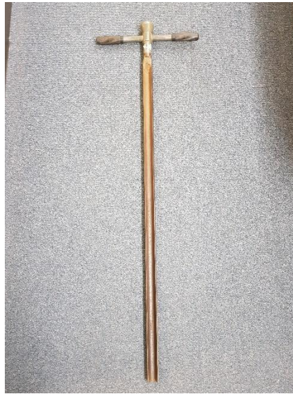
Figure 2.2: 25 mm gauge corer used for extracting cores of the Waulkmill Bay and Loch of Stenness saltmarshes.
