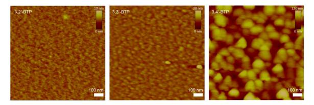
**Figure S2** | Atomic force micrograph of BTPs evaporated as 40 nm thick films onto Si-wafer. 3,2'- and 3,3'-BTP deposit as flat films, while 3,4'-BTP deposits as islands that grow into globes.
