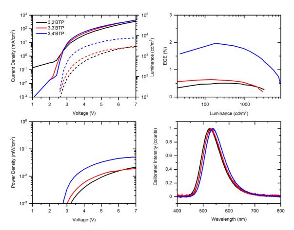
**Figure S20** | (a) Current density and luminance plotted against the applied voltage of the bottom-emitting OLEDs. (b) External quantum efficiency in % plotted against luminance. (c) Power density versus voltage. (d) Normalized electroluminescence spectra. All data color-coded with 3,2'BTP (black), 3,3'BTP (red) and 3,4'BTP (blue).
