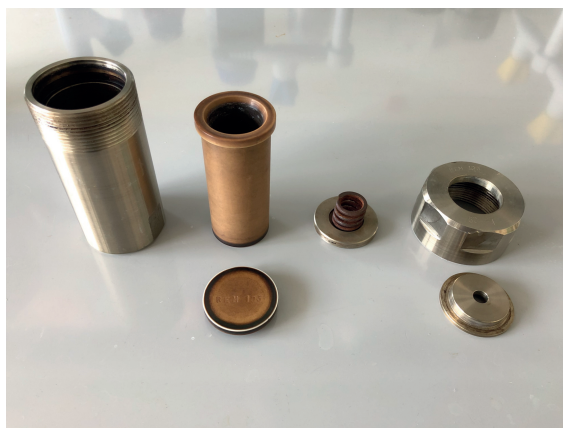
Figure 1.5: Components of an autoclave used in hydrothermal zeolite synthesis. Left to right, steel body, Teflon liner and lid, steel blast ring, steel plate and lid.
