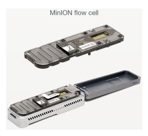
**Figure 3.2: The MinION sequencing platform.** A small-form sequencer released by Oxford Nanopore Technologies (ONT), showing the flowcell [*top*] where the DNA/RNA library is loaded. The flowcell contains 2048 individual nanopores through which the DNA strand passes to allow sequencing. The flow cell is inserted into the MinION [*bottom*] which provides power to maintain a set temperature and voltage via USB connection to a computer [16].
