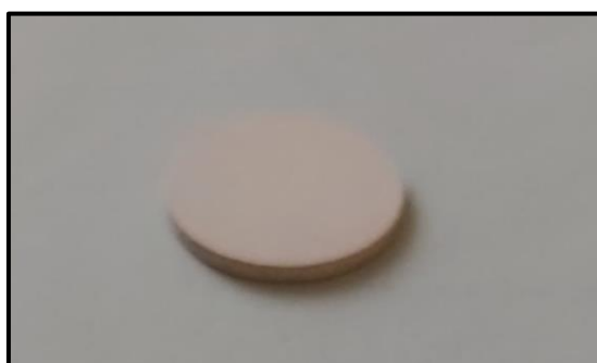
Figure 2.1: Ceramic pellet of \text{LaTaO}_4 ~10 mm diameter pressed at 30,000 psi and heated to 1923 K for 6 hrs. Theoretical density \approx 75%.
