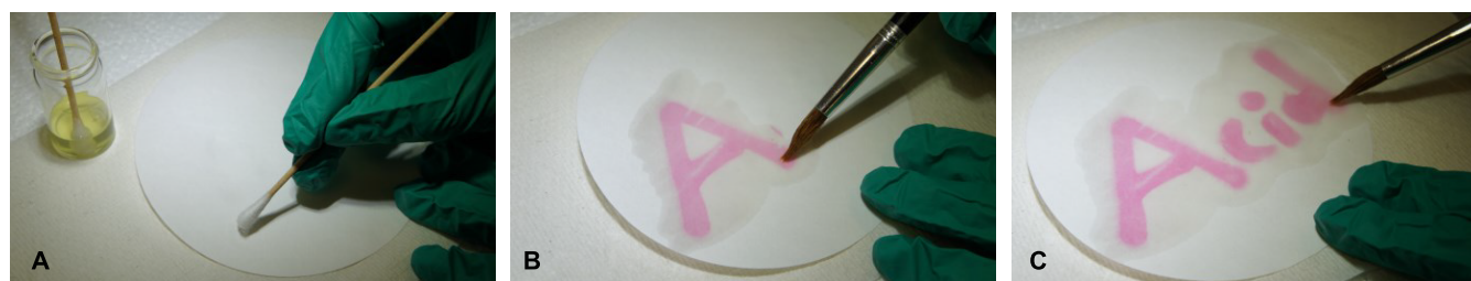
Figure 3. Revealing hidden messages written using bleached anthocyanin solution. Step A: Writing a message on filter paper using a cotton swab dipped in the bleached solution. Steps B and C: Application of 10% citric acid solution with a paint brush to reveal the hidden message.
