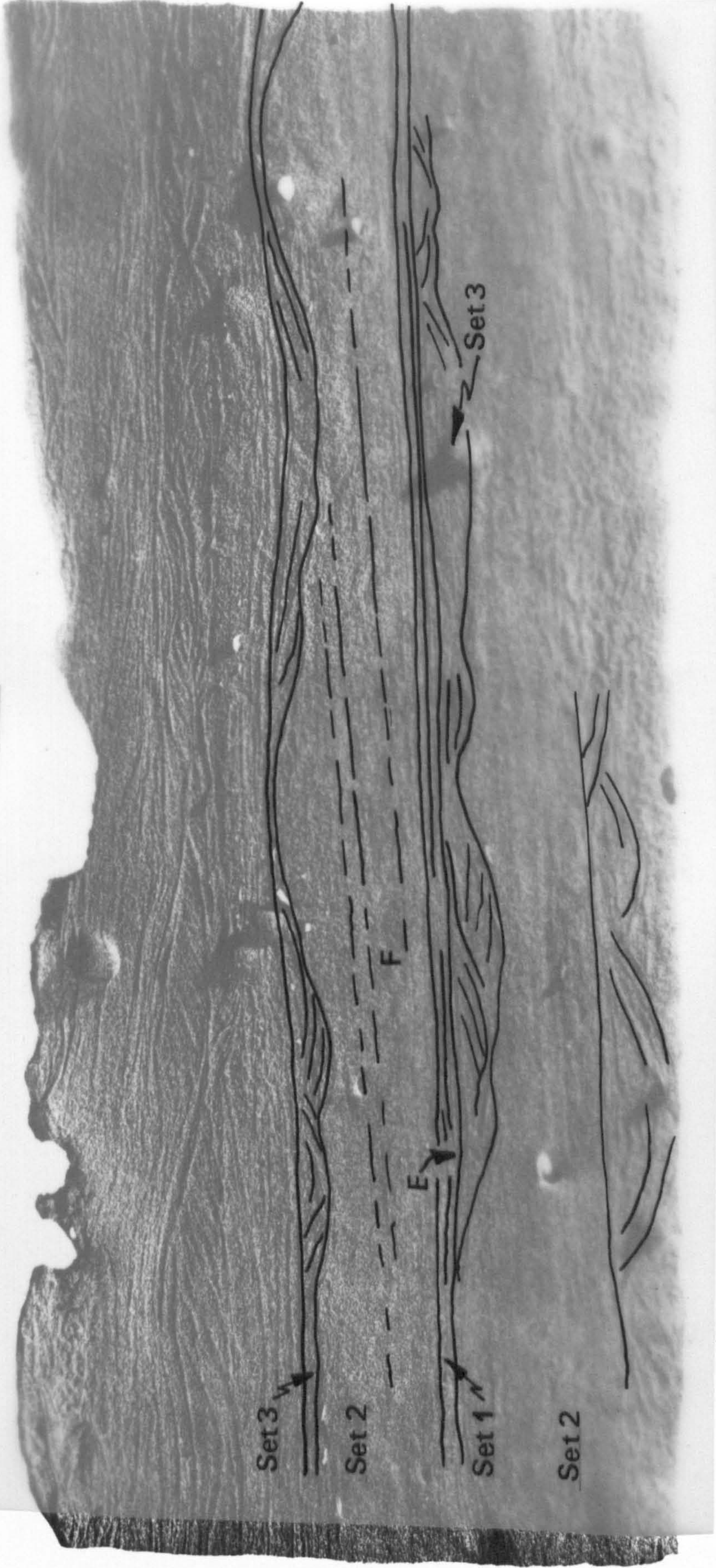
Fig. 3.35. Epoxy resin peel, perpendicular to flow direction, of structures in the same sand-wave as in Fig. 3.34.
