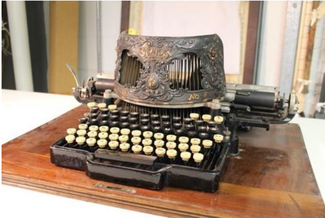
Figure 4.19. Bar-Lock No. 5 was manufactured in c. 1893 for the British market. The typebars are arranged upright in front of the carriage. NMS collection, object number T.1959.41.
