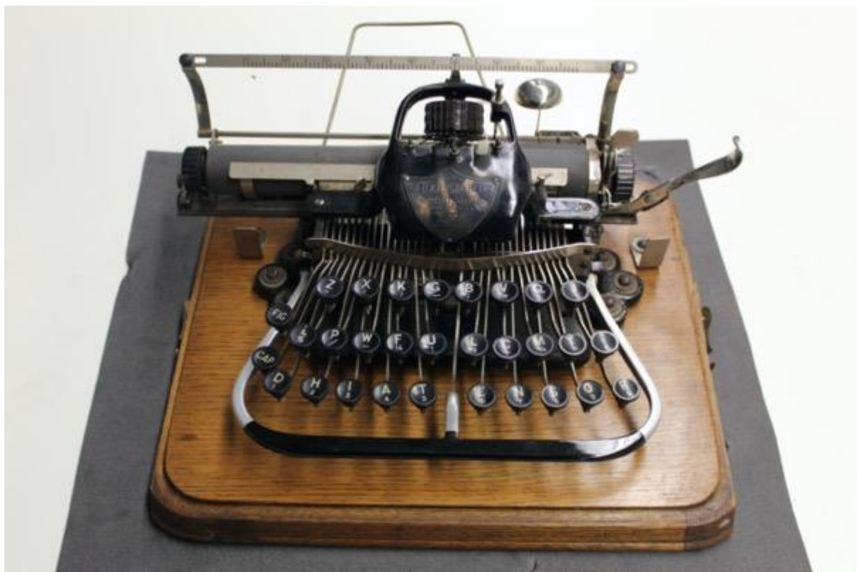
Figure 1.10. Blickensderfer No. 7 typewriter with Scientific Keyboard. In object handling collection at NMS.
