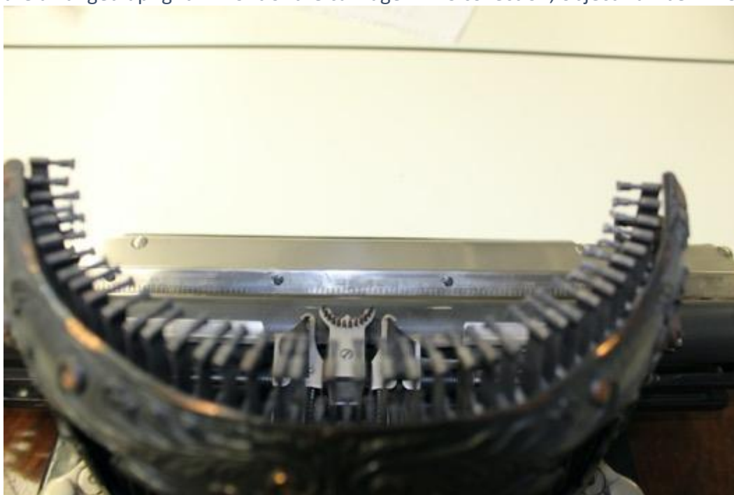
Figure 4.20. Typist's vantage point over the typebars down onto the printing point on the Bar-Lock No. 5.
