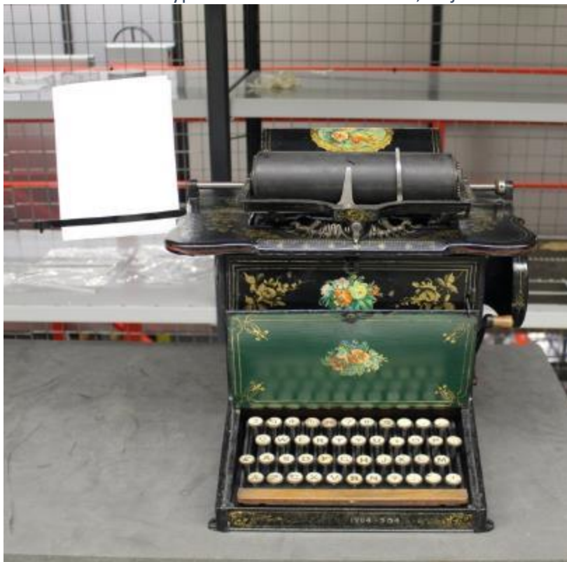
Figure 4.8. Sholes & Glidden typewriter, c. 1876, with copyholder and side lever for carriage return. NMS collection, object number T.1904.304.
