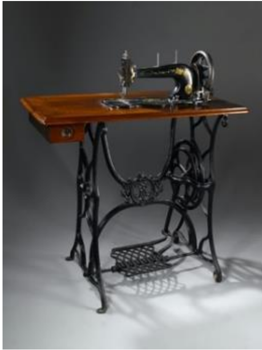
Figure 4.7. Frister & Rossman sewing machine c. 1870. The cast-iron stand, the treadle and decals were design elements that featured on early Sholes & Glidden typewriters. NMS collection, object number T.1960.66.
