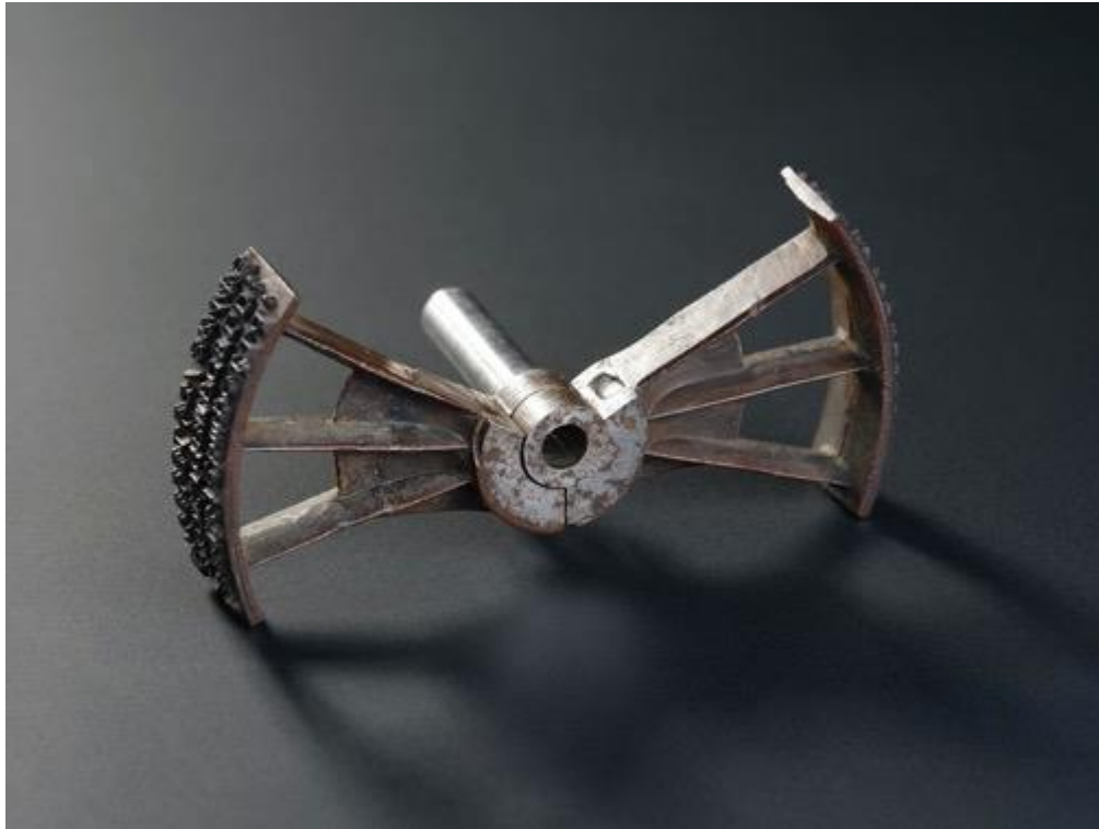
Figure 5.15. Interchangeable type segment for use on Hammond typewriters. This design made Hammond typewriters much lighter and more portable than Remingtons which had separate metal typebars for each key. NMS collection, object number T.1934.182.2
