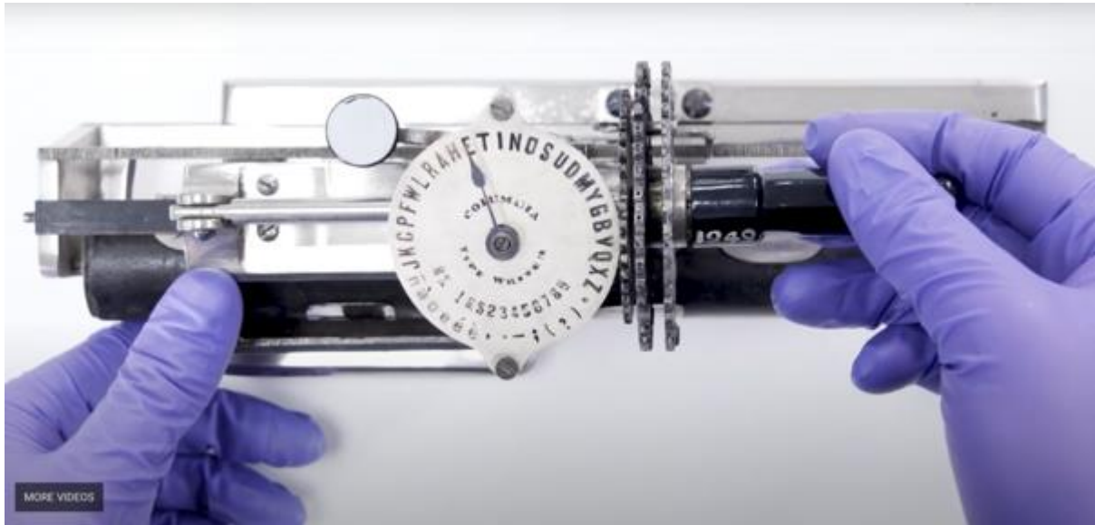
Figure 1.1. Demonstration of Columbia No. 2 typewriter made in New York, c. 1885. NMS collection, object number T.1949.3.1. For video demonstration visit: https://www.nms.ac.uk/explore-our-collections/stories/science-and-technology/history-of-the-typewriter/
