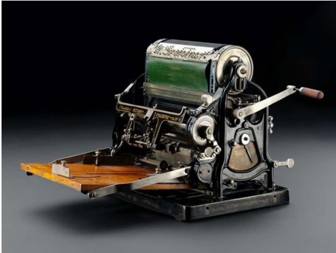
Figure 5.16. Gestetner duplicator, the 'Rotary Cyclostyle No 6', made in London, c. 1910. Held in NMS collection, object number. T.1979.X.57.
